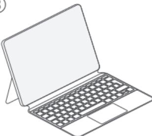
Note: The keyboard will only enter operating mode once the Pad and keyboard have been linked together correctly as shown above.
